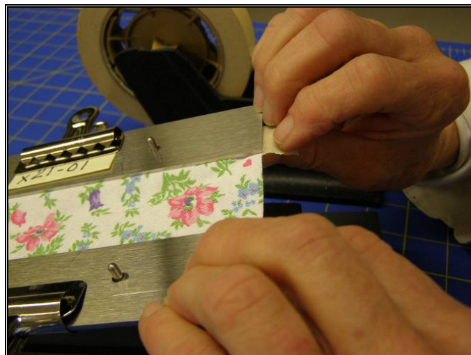
Figure 9. Tape may be used to further secure specimen.
