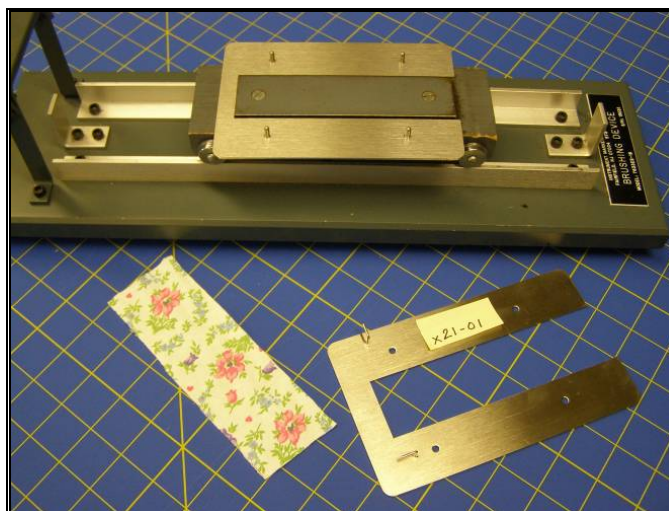
Figure 4. Place back plate of specimen holder on brushing device carriage.
