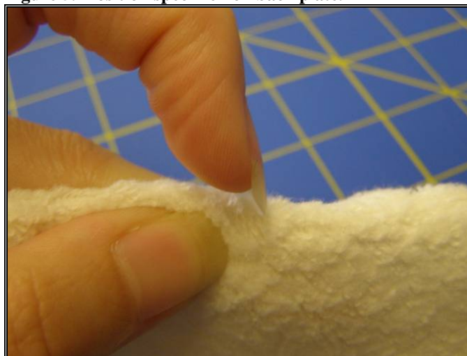
Figure 6. Determine the lay of the pile.
