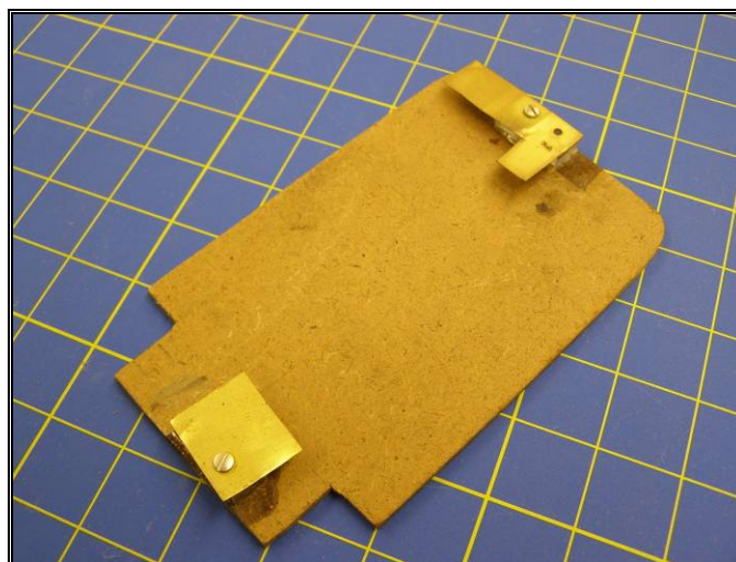
Figure 34. Example calibration plate for timer.
